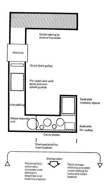
Appendix XV Diagrammatic Layout Suitable for Central Crockery Wash in Medium Size Hospitals
